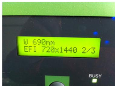
The printer control panel in the image above shows that the printer is currently printing layer two out of a total of three.
